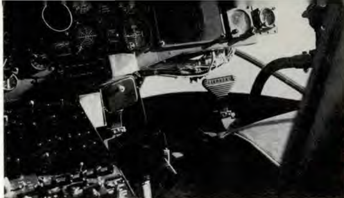
The right side of an HH-53 cockpit showing the NRS equipment installation.
