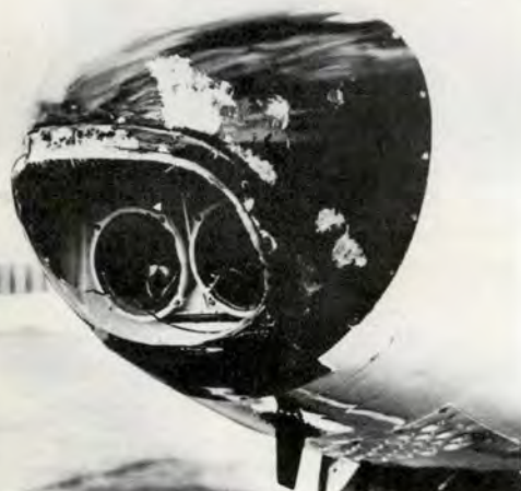
T-39 (above) and B-52 show damage sustained in hail encounters. Hail, ice, water, intensive up and down drafts are characteristic of well developed T-storms.
