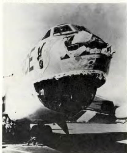
T-39 (above) and B-52 show damage sustained in hail encounters. Hail, ice, water, intensive up and down drafts are characteristic of well developed T-storms.
